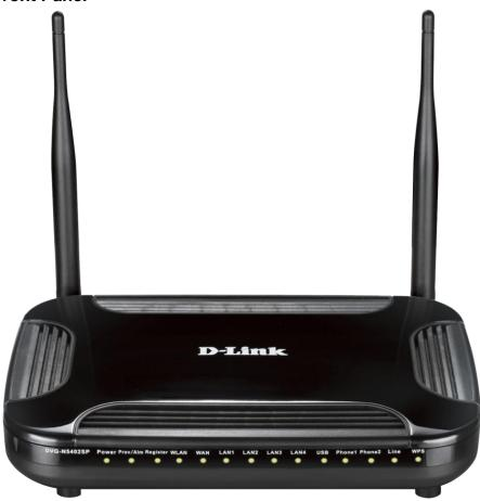
**Power**: A steady green light indicates a proper connection to a power source. A red light indicates the power-on self test fails or the device is malfunction.
